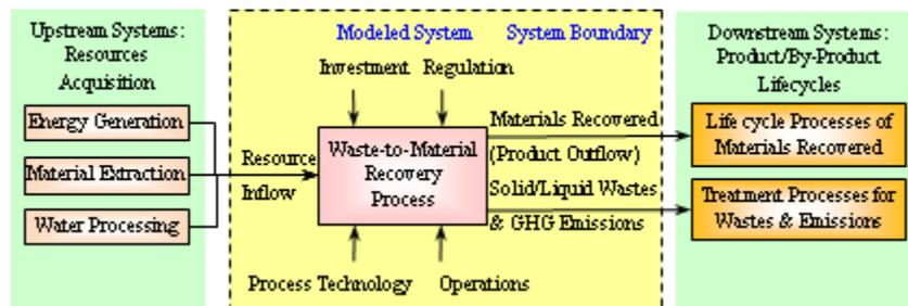
Figure 4. Boundary setting for metrics modeling of waste-to-material recovery processes.
