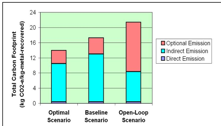
Figure 13. Comparison of carbon footprints of two recovery technologies for three scenarios.
