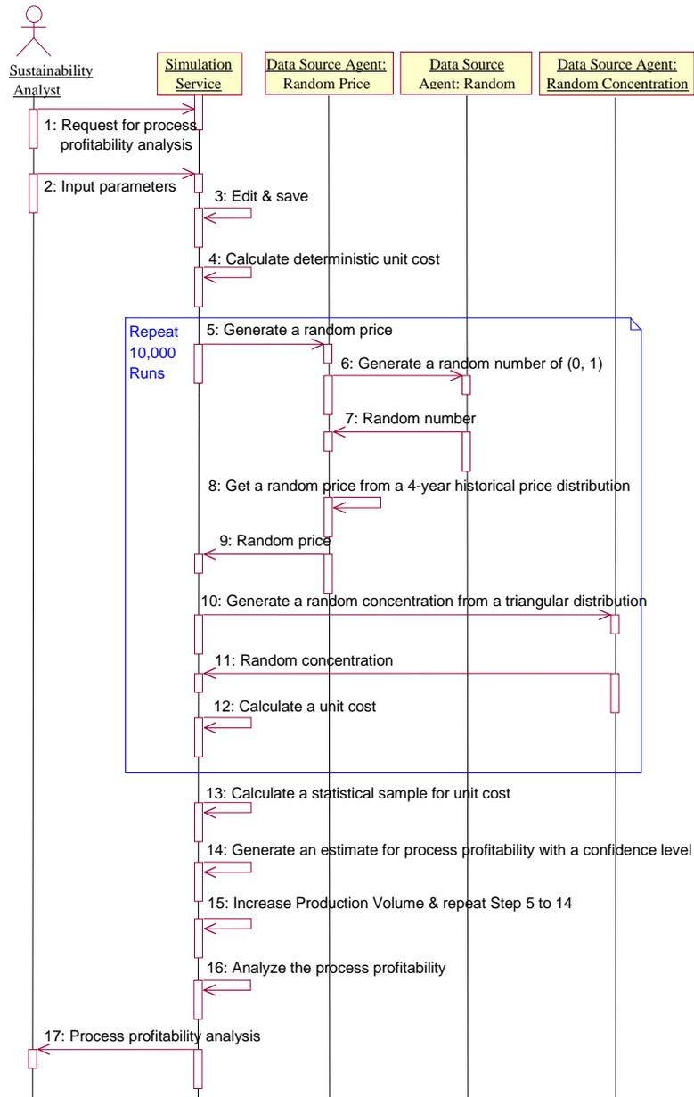
Figure 8. Sequence diagram for probabilistic analysis of *process profitability*.
