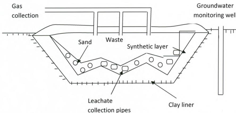
Figure 2.4: Cross section of a typical municipal solid waste landfill (Source: Masters and Ela, 2008)
