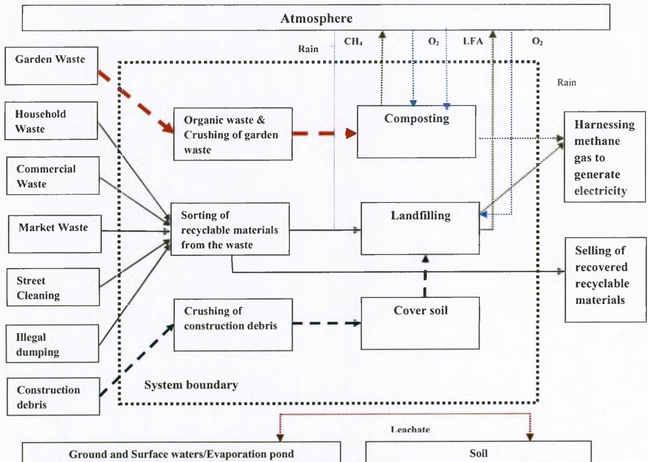
Figure 4.4: System analysis of solid waste material stream through Robinson Deep Landfill (Author, 2015)
