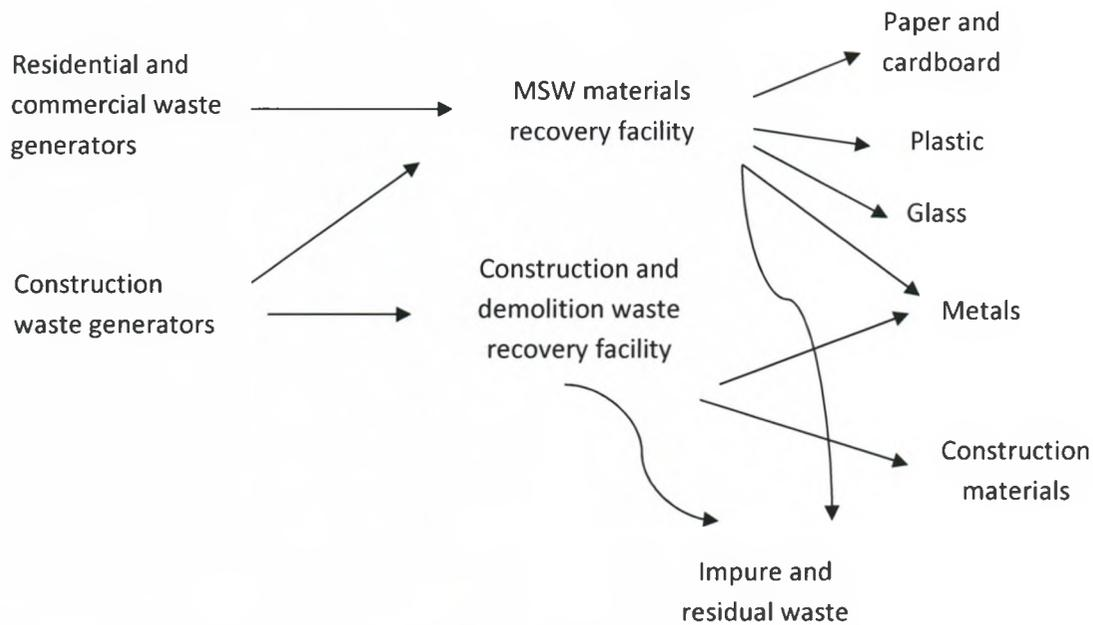
Figure 2.3: A recycling system including the waste generators, material recovery facilities, and markets for recovered material (Source: Mihelcic and Zimmerman, 2010)
